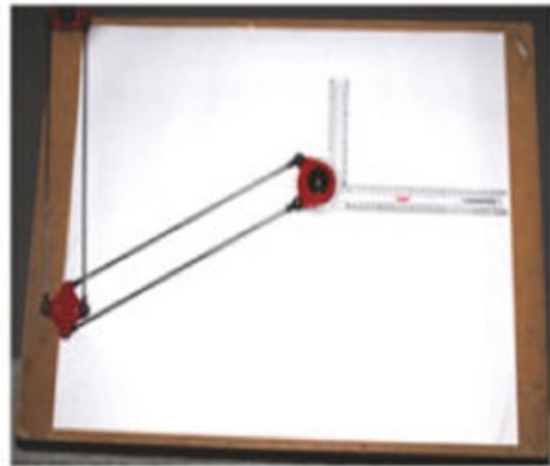
Photograph of a typical college level drawing table, drawing board and mini-drafter assembly
